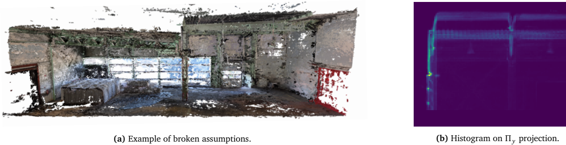
Figure 5: Scene 7 reconstruction, where our axis-aligned assumptions fail partially on one axis projection, due to the roof being formed of two parallel sections.
